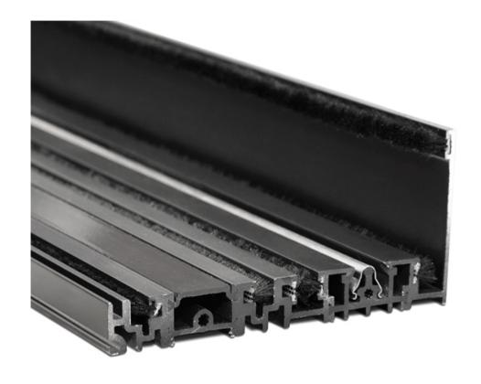
The Series 7650 Sliding Glass Door comes standard with a 1.5" sill. For increased effectiveness against the elements, 2" and 2.6" options feature a higher interior leg. The 1.5", 2", and 2.6" sills meet the commercial specifications of the American Architectural Manufacturers Association (AAMA) and boast a performance rating of DP50. A flush sill option that lines up with most interior flooring is also available. All sills are finished to match the color of the frame.
