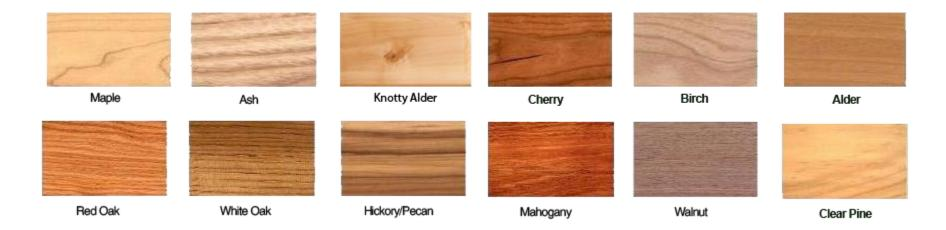
**Alder:** Alder is a relatively soft hardwood of medium density that has low bending strength, shock resistance, and stiffness. Alder, a relative of birch, is almost white when freshly cut, but quickly changes with exposure to air, becoming light brown with a yellow or reddish tinge. Heartwood is formed only in trees of advanced age and there is no visible boundary between sap and heartwood. The wood is fairly straight-grained with a uniform texture.
